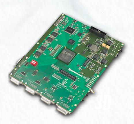
RealityBox is a real-time image and video conversion hardware platform for creating stereoscopic (S-3D) or auto-stereoscopic (AS-3D) content from monoscopic (2D) or stereoscopic (S-3D) source content. RealityBox is a prototype implemented on a Lattice ECP3 to show the full functional conversion capabilities. More cost efficient solutions can be generated out of the existing IP depending on the customer requirements.
